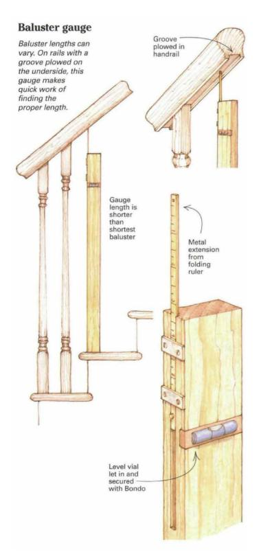
Spindle-hole sizing gauge
