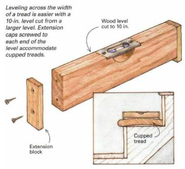
When leveling treads from front to back, it's handy to have a small level. You could buy a small bullet level, but I've never found one that didn't seem like a toy. I cut down a larger wood level to 10 in. and screwed small extension blocks of wood on the ends. The blocks extend past the bottom of the level because sometimes a tread isn't exactly flat, so the extension blocks allow the body of the level to clear the belly of a chubby tread and
