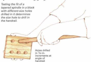
The diameter of the top, or thin end, of a tapered spindle can decrease as the spindle gets longer. Therefore, the hole drilled into the handrail for the back spindle on a tread can be smaller than the hole for the front baluster.
