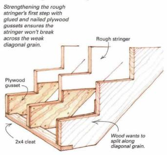
Often, because the carriage at the first tread must be cut shorter than the unit rise to allow for tread thickness (usually 1 in.) and also notched for a 2x4 floor cleat, the bottom of the carriage is weakened. I always beef up the carriages by screwing and gluing a piece of plywood to the sides.
